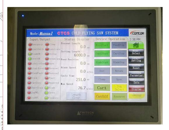
After finishing the above procedures, press orderly the buttons of feeding on, blade on and cart on and clamps on to make the machine cut in the condition of no pipes and observe if everything for cutting is normal.
